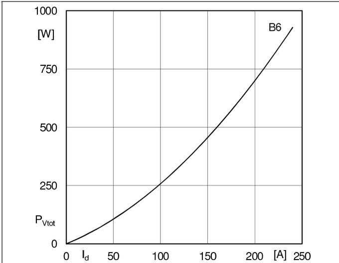
Fig. 4L: Power dissipation per module vs. direct current
