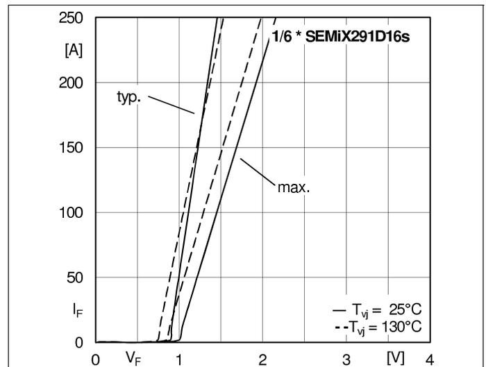
Fig. 7: On-state characteristics
