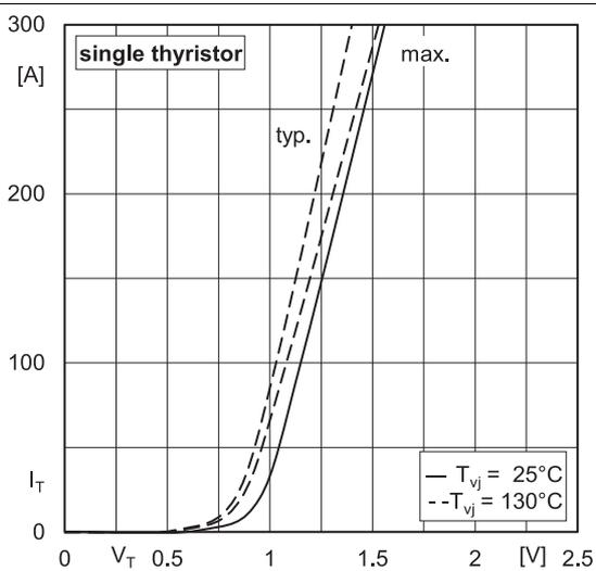
Fig. 7: On-state characteristics
