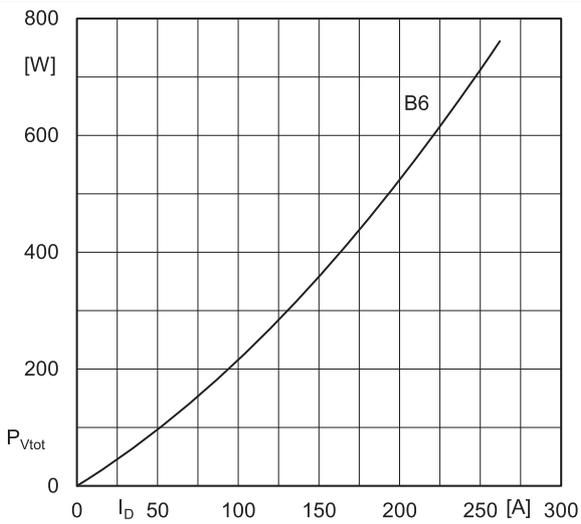
Fig. 4L: Power dissipation per module vs. direct current
