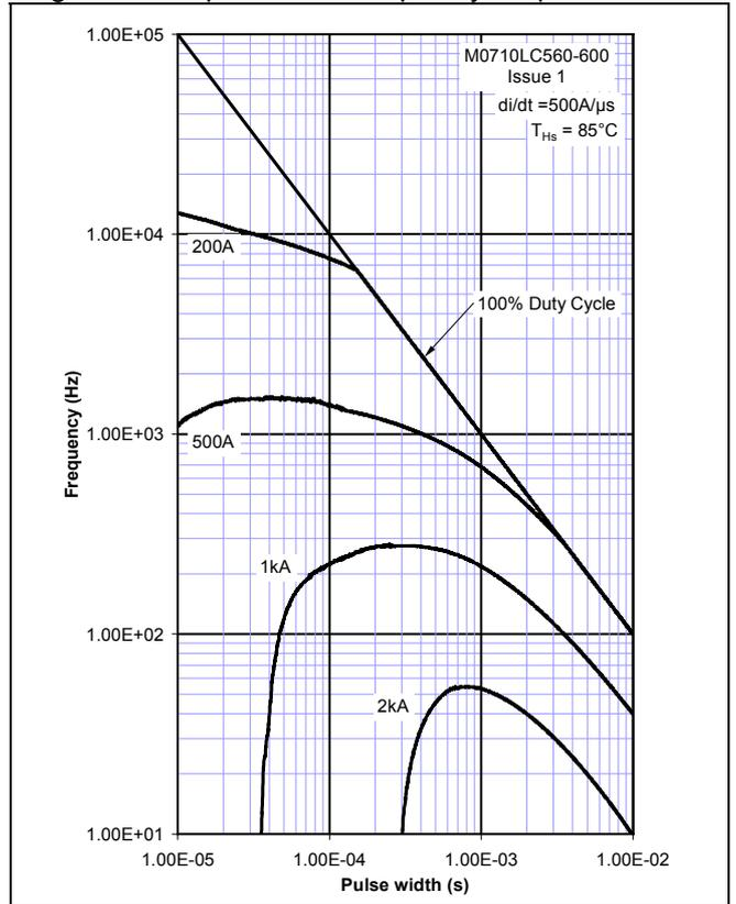
Figure 15 - Square wave frequency vs. pulse width
