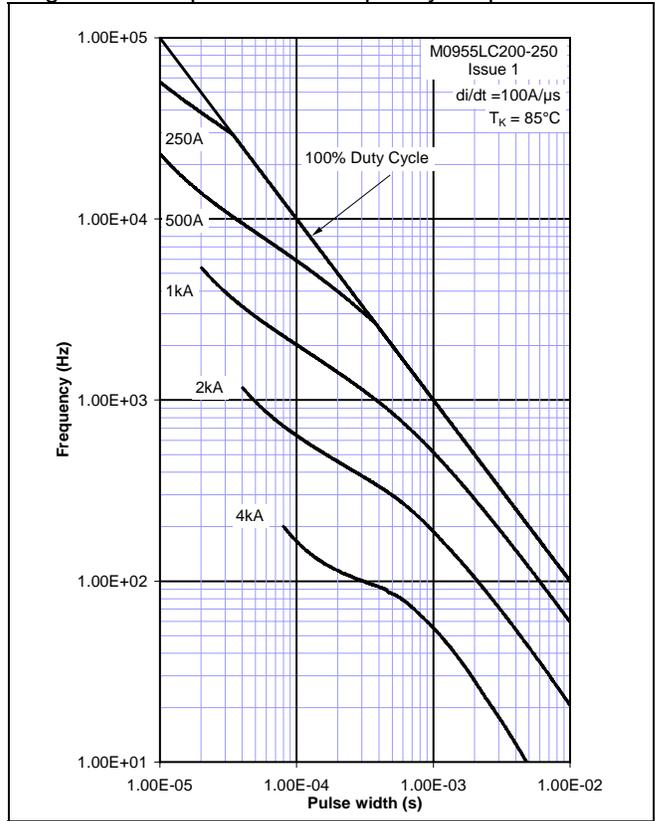
Figure 15 – Square wave frequency vs. pulse width
