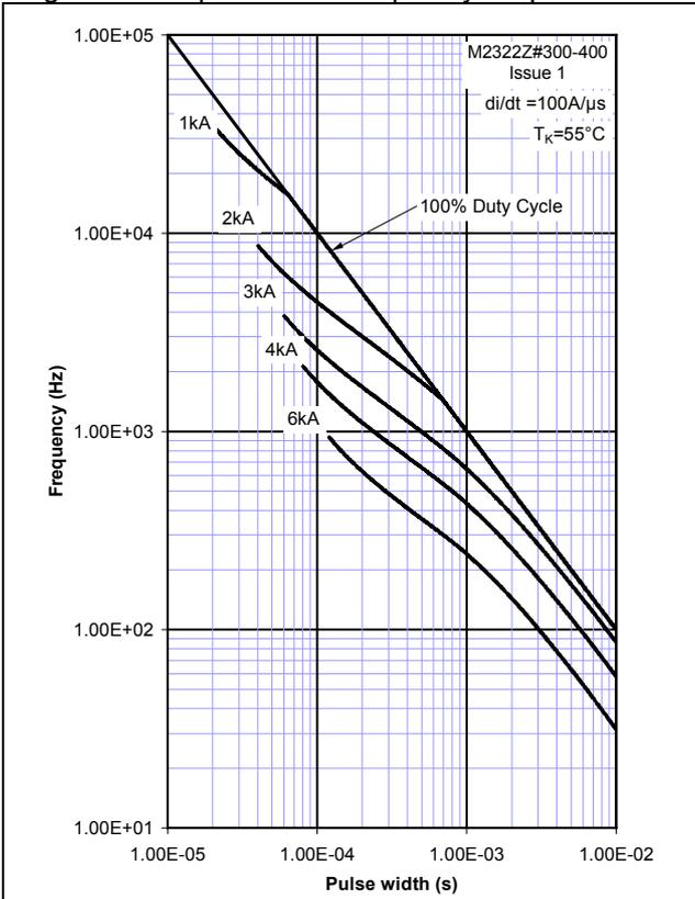
Figure 12 - Square wave frequency vs. pulse width
