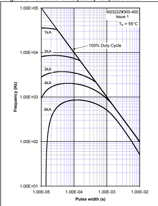
Figure 10 - Sine wave frequency vs. pulse width
