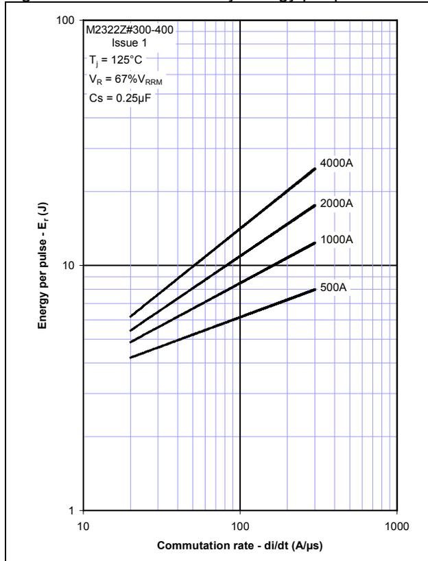
Figure 8 - Sine wave energy per pulse
