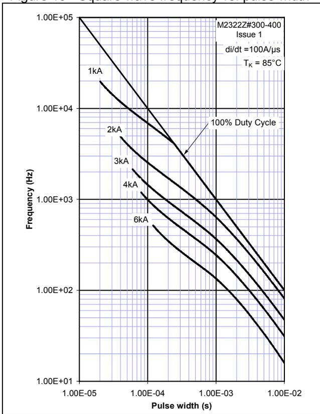
Figure 14 - Square wave frequency vs. pulse width
