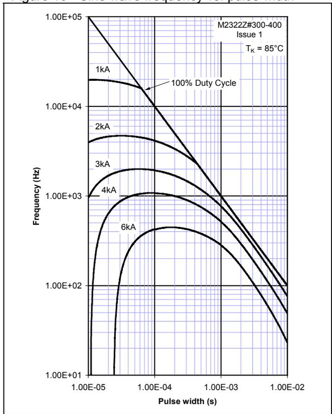
Figure 11 - Square wave frequency vs. pulse width
