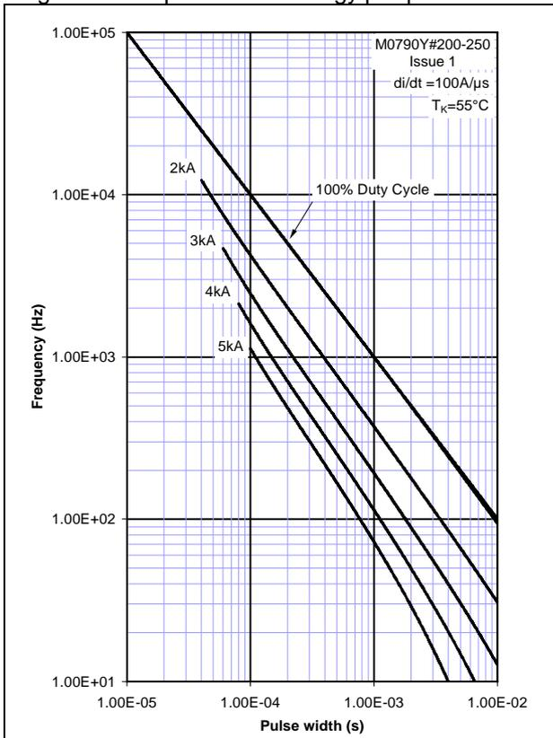
Figure 12 - Square wave energy per pulse
