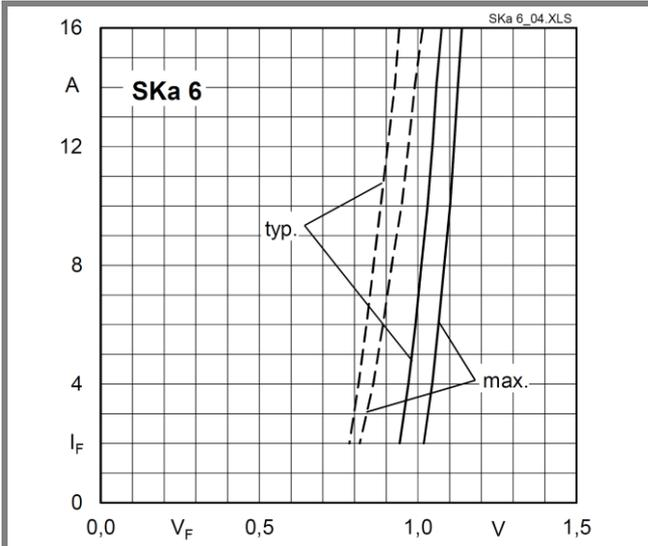
Fig. 6 Forward characteristics
