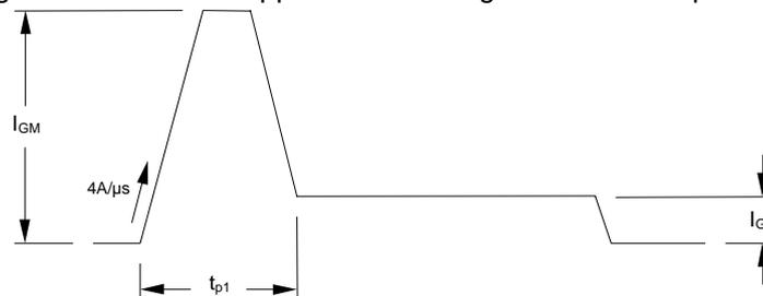
The magnitude of  $I_{GM}$  should be between five and ten times  $I_{GT}$ , which is shown on page 2. Its duration ( $t_{p1}$ ) should be 20 $\mu$ s or sufficient to allow the anode current to reach ten times  $I_L$ , whichever is greater. Otherwise, an increase in pulse current could be needed to supply the necessary charge to trigger. The 'back-porch' current  $I_G$  should remain flowing for the same duration as the anode current and have a magnitude in the order of 1.5 times  $I_{GT}$ .
