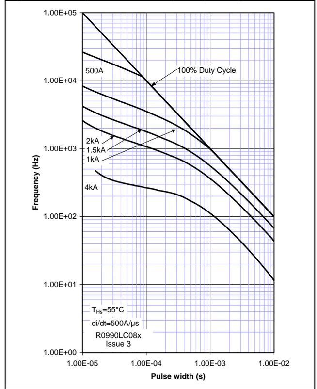
Figure 15 - Square wave frequency ratings
