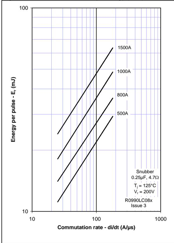
Figure 10 - Sine wave energy per pulse
