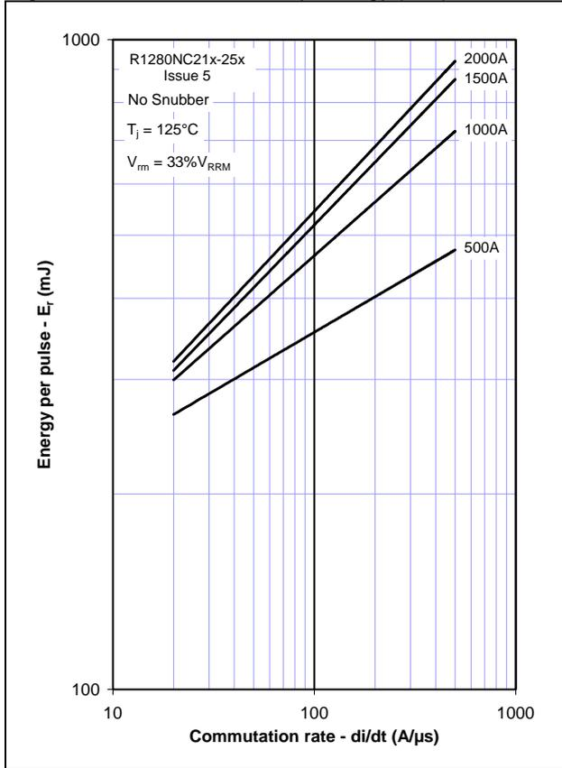
Figure 10 - Sine wave energy per pulse
