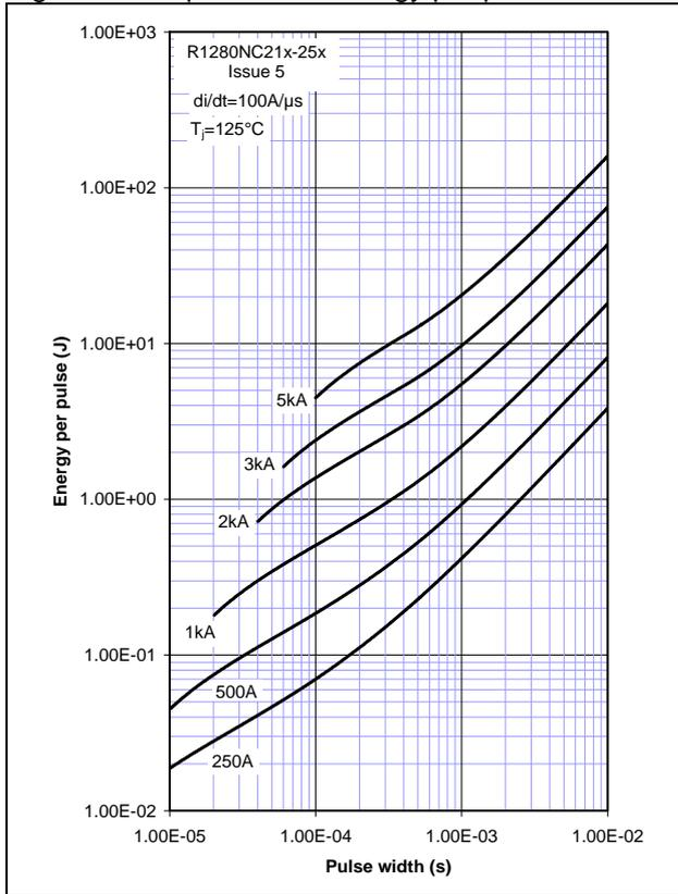
Figure 18 - Square wave energy per pulse
