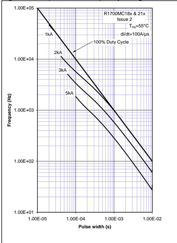
Figure 14 - Square wave frequency ratings
