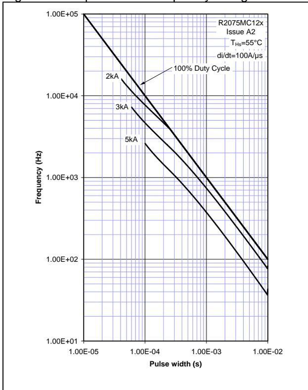
Figure 14 - Square wave frequency ratings
