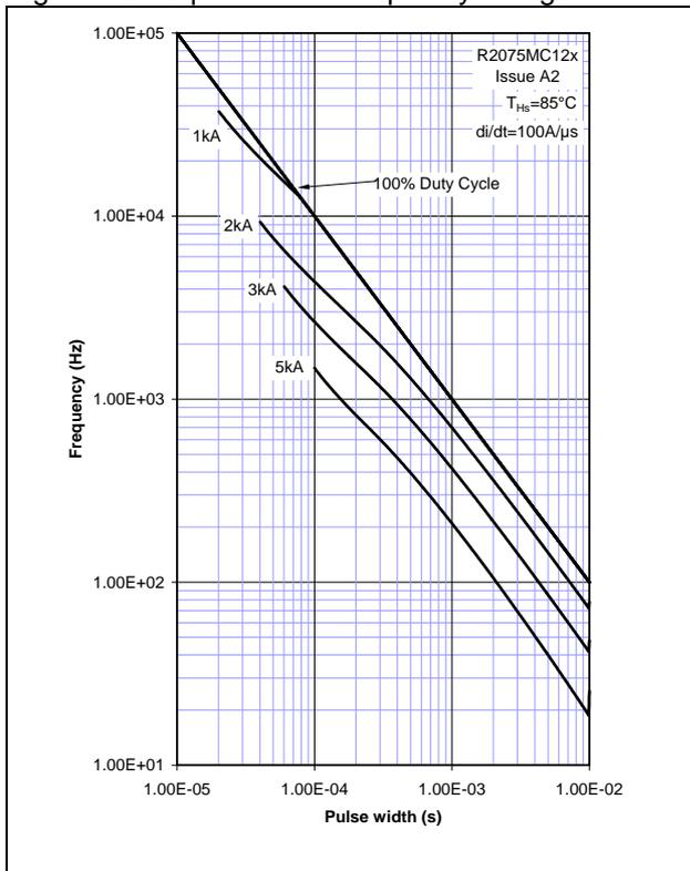
Figure 16 - Square wave frequency ratings
