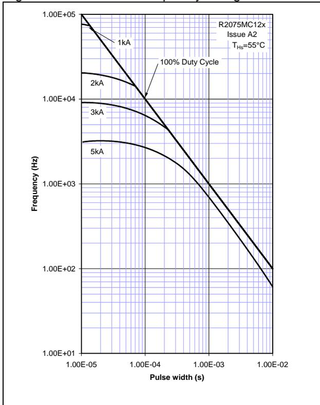
Figure 12 - Sine wave frequency ratings
