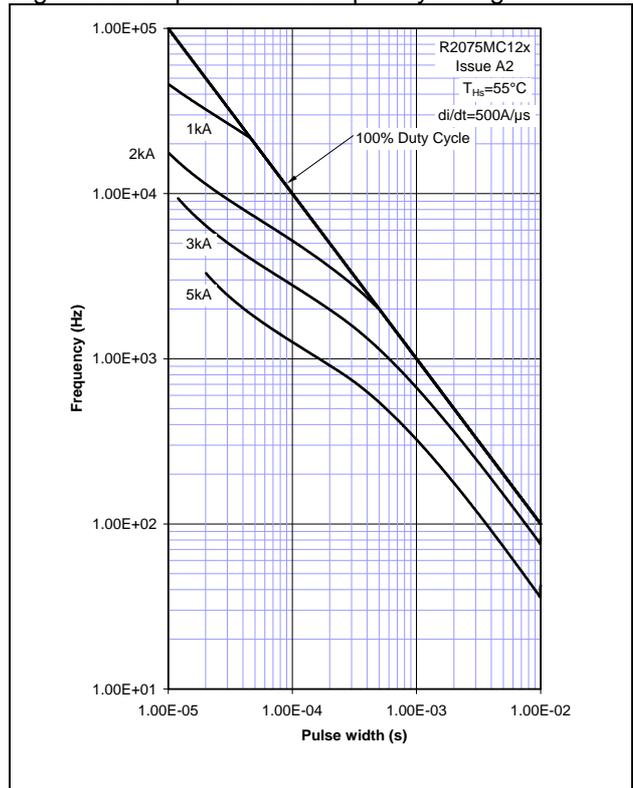
Figure 15 - Square wave frequency ratings
