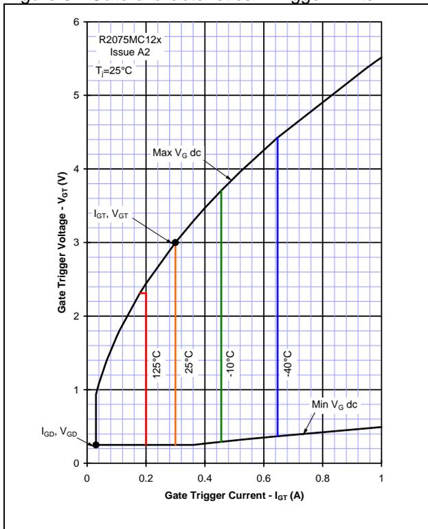
Figure 4 - Gate characteristics - Power curves
