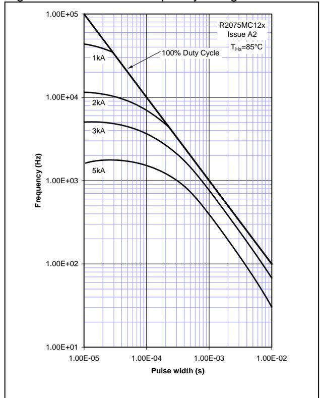
Figure 13 - Square wave frequency ratings
