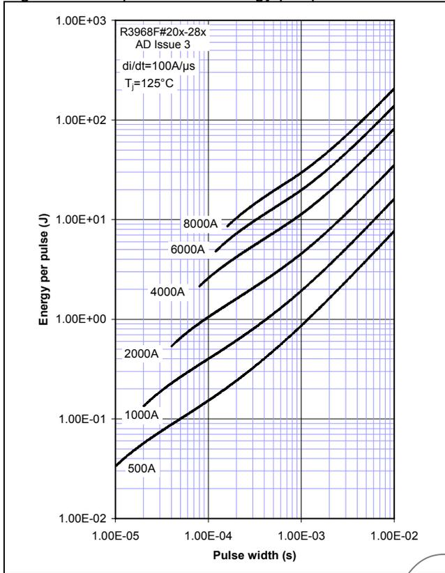
Figure 18 – Square wave energy per pulse
