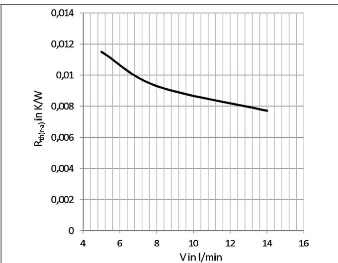
Fig. 9: Thermal resistance  $R_{th}(r-a)$  versus flow rate  $V$
