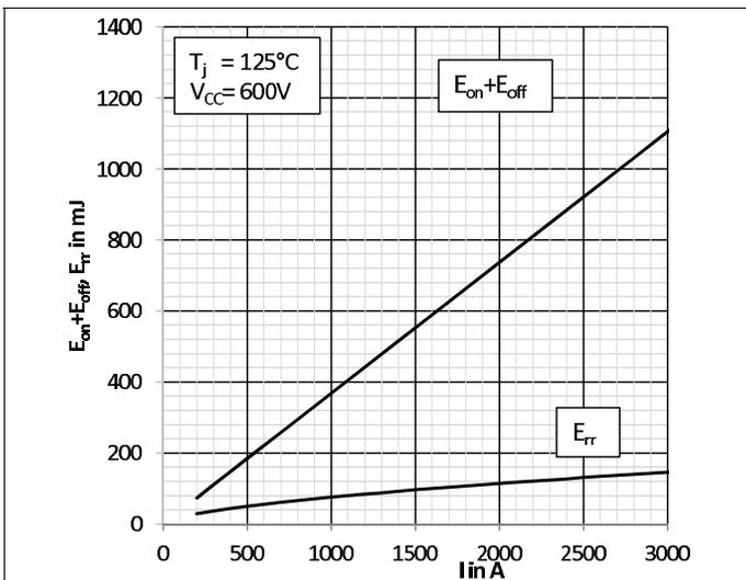
Fig. 3: Typical energy losses  $E = f(I_C, V_{CC})$
