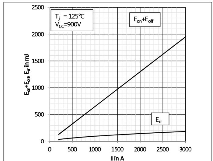
Fig. 4: Typical energy losses  $E = f(I_C, V_{CC})$
