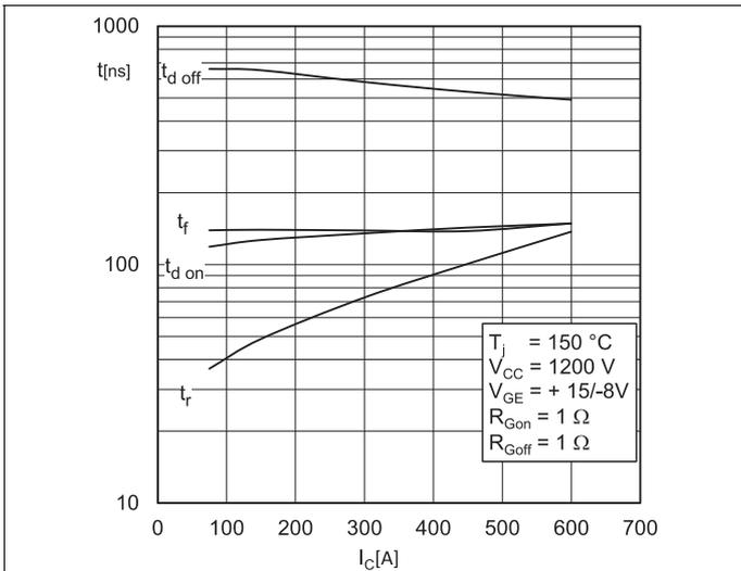
Fig. 7: Typ. IGBT1 switching times vs.  $I_C$
