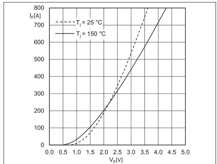
Fig. 10: Typ. Diode2 forward characteristic, incl.  $R_{CC+EE'}$
