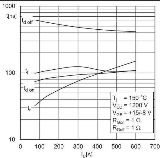
Fig. 19: Typ. IGBT2 switching times vs.  $I_C$
