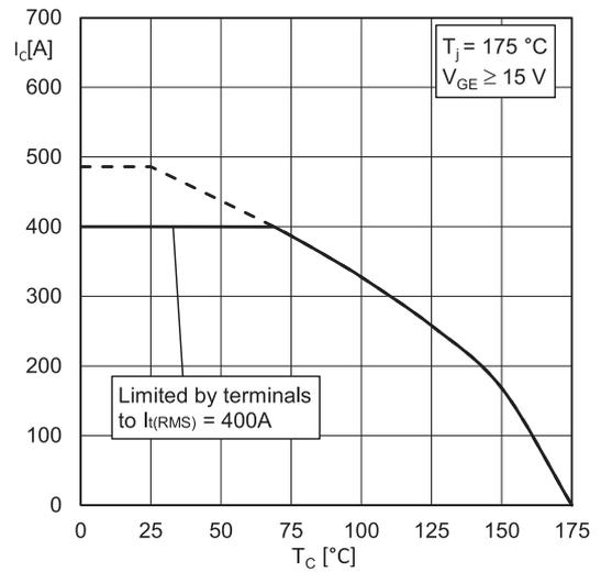
Fig. 2: IGBT1 rated current vs. Temperature  $I_C=f(T_C)$
