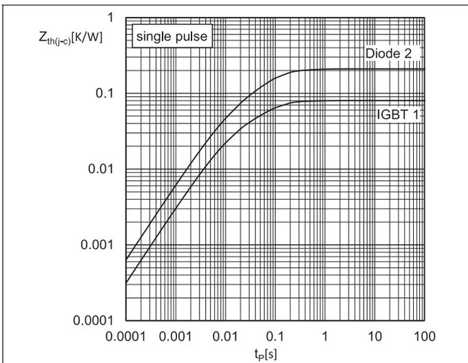
Fig. 9: Transient thermal impedance of IGBT1 & Diode2
