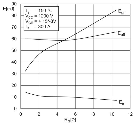
Fig. 4: Typ. IGBT1 & Diode2 turn-on /-off energy =  $f(R_G)$
