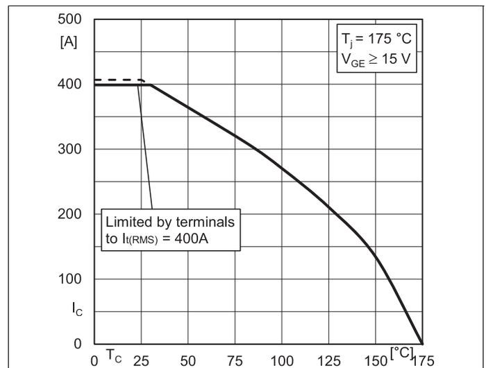
Fig. 14: IGBT2 Rated current vs. Temperature  $I_C = f(T_C)$
