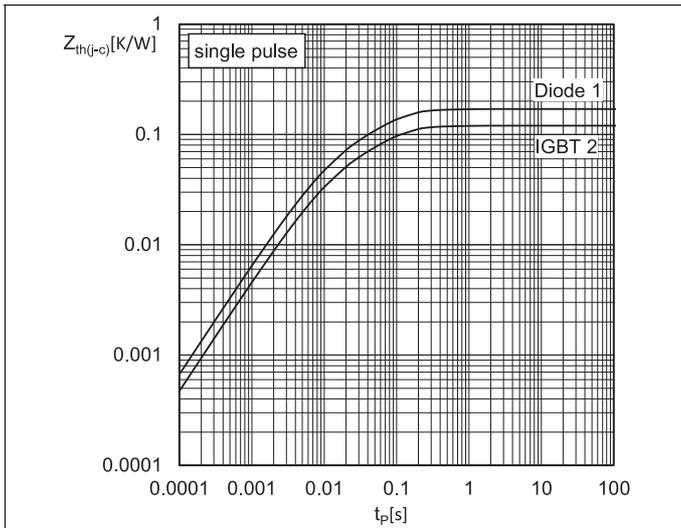
Fig. 21: Transient thermal impedance of IGBT2 & Diode1
