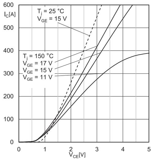
Fig. 1: Typ. IGBT1 output characteristic, incl.  $R_{CC'+EE'}$
