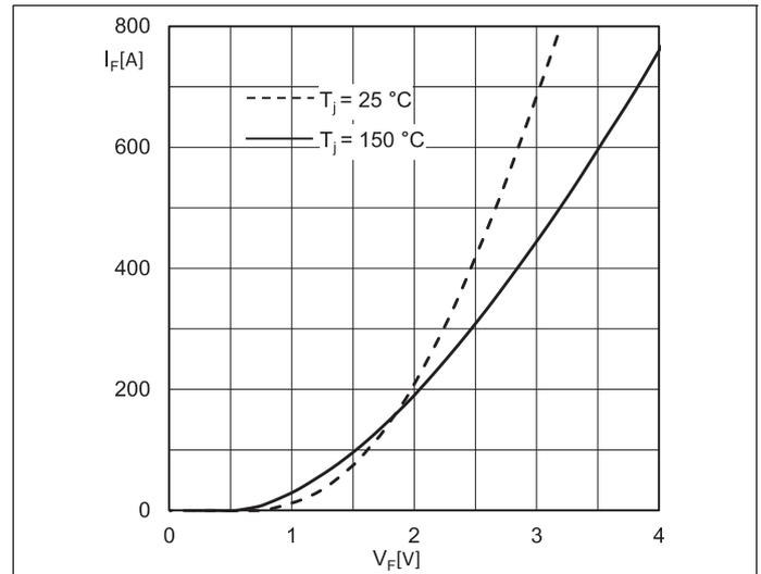
Fig. 22: Typ. Diode1 forward characteristic, incl.  $R_{CC'+EE'}$
