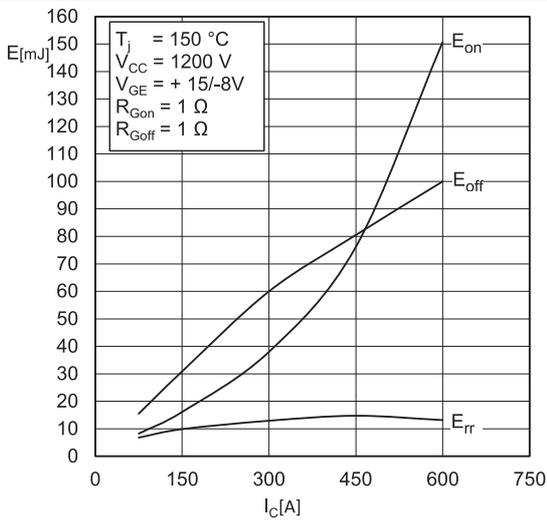
Fig. 3: Typ. IGBT1 & Diode2 turn-on /-off energy =  $f(I_C)$
