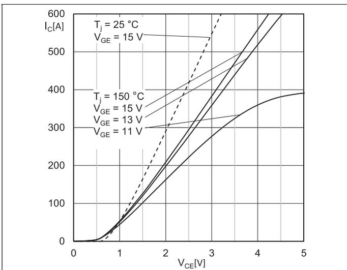
Fig. 13: Typ. IGBT2 output characteristic, incl.  $R_{CC+EE'}$
