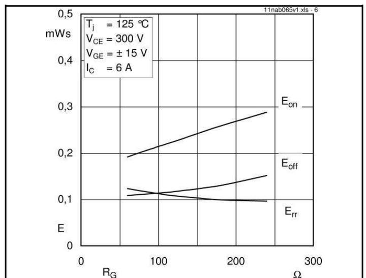
Fig. 6 Typ. Turn-on /-off energy =  $f(R_G)$
