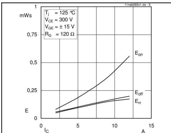
Fig. 5 Typ. Turn-on /-off energy =  $f(I_C)$
