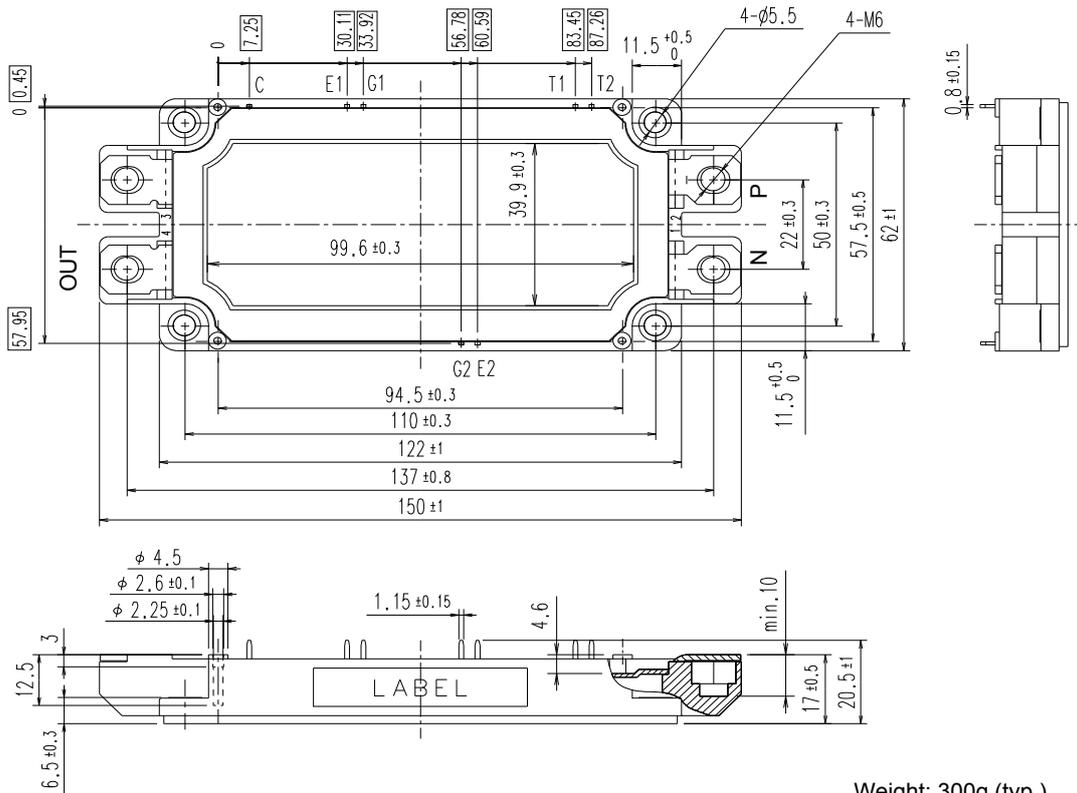
NOTE)   shows theoretical dimension and tolerance is  $\pm \phi 0.5$
