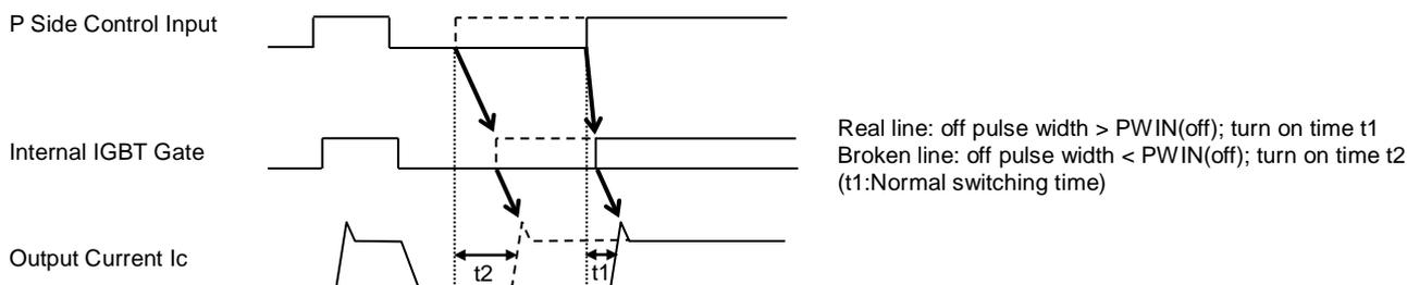
Fig. 5 Timing Charts of The DIIPM Protective Functions
