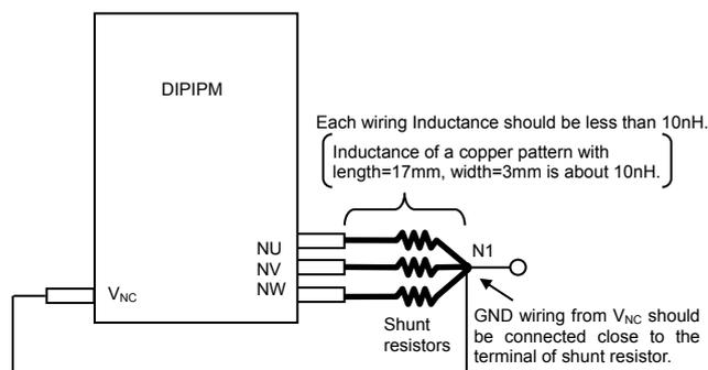
Low inductance shunt resistor like surface mounted (SMD) type is recommended. Protection current level I<sub>sc</sub> changes by inserting shunt resistor.
