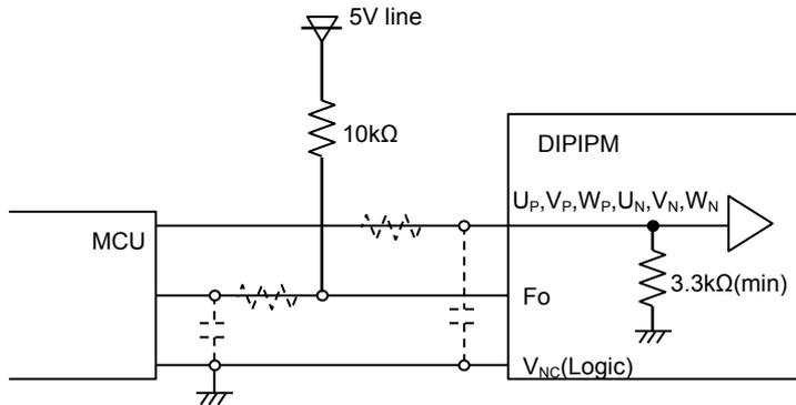
Note: The RC coupling (parts shown in the dotted line) at each input depends on user's PWM control strategy and the wiring impedance of the printed circuit board. The DIIPM signal input section integrates a 3.3kΩ(min) pull-down resistor. Therefore, when using an external filtering resistor, please pay attention to the signal voltage drop at input terminal.
