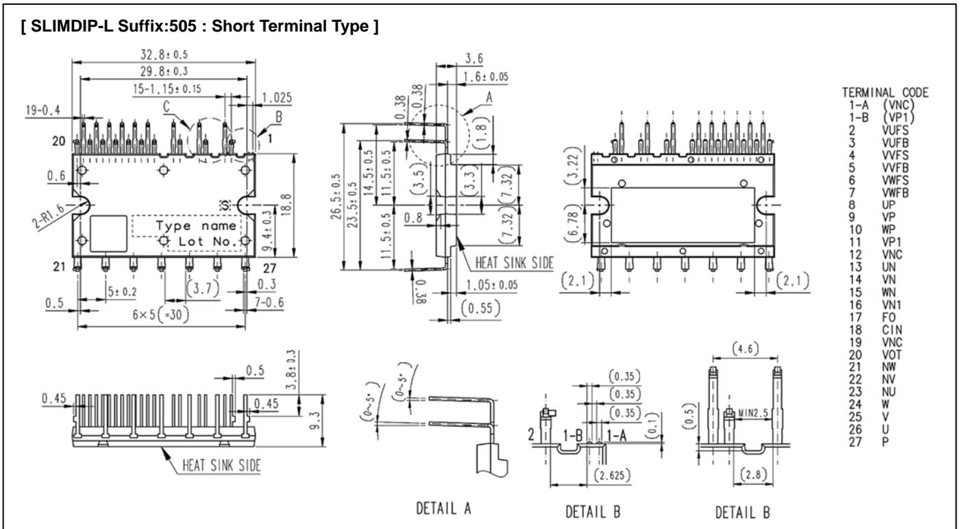
Note: Connect only one V<sub>NC</sub> terminal (No.12 or 19) to the system GND and leave another one open.
