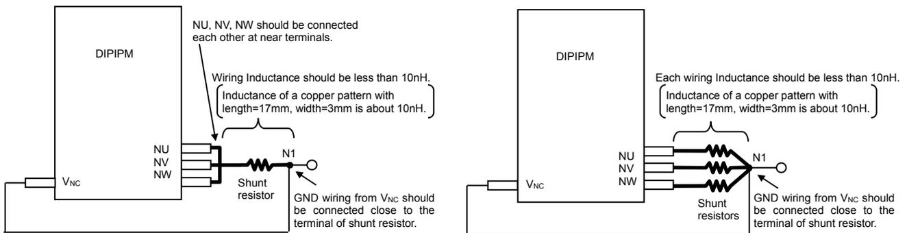
Low inductance shunt resistor like surface mounted (SMD) type is recommended.
