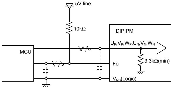
Note: The RC coupling (parts shown in the dotted line) at each input depends on user's PWM control strategy and the wiring impedance of the printed circuit board. The DIIPIM signal input section integrates a 3.3kΩ(min) pull-down resistor. Therefore, when using an external filtering resistor, please pay attention to the signal voltage drop at input terminal.
