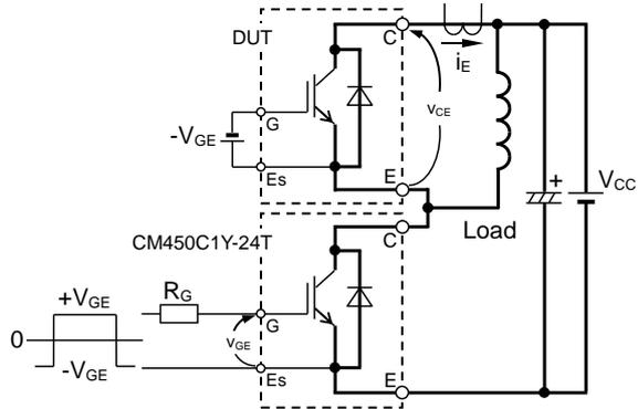
$t_{rr}$ ,  $Q_{rr}$  characteristics test circuit and waveform
