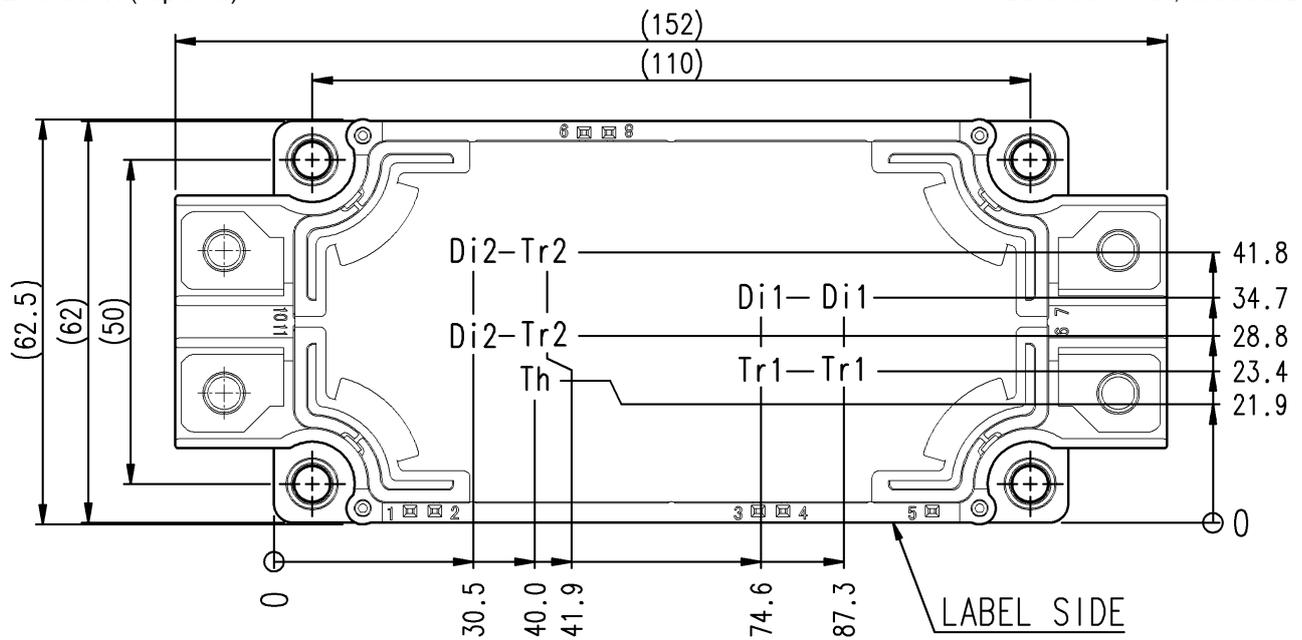
Tr1/Tr2: IGBT, Di1/Di2: FWD, Th: NTC thermistor
