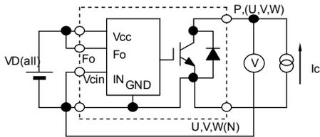
Fig.1  $V_{CESat}$  Test
