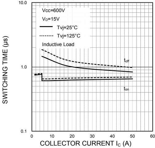
SWITCHING TIME ( $t_{c(on)}$ ,  $t_{c(off)}$ ) CHARACTERISTICS (TYPICAL)
