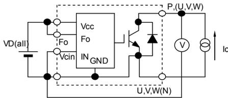
Fig.1  $V_{CESat}$  Test
