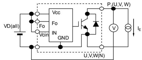
Fig.2  $V_{EC}$  Test
